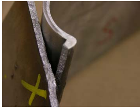
Figure 12. Failed weld; no ductility.
