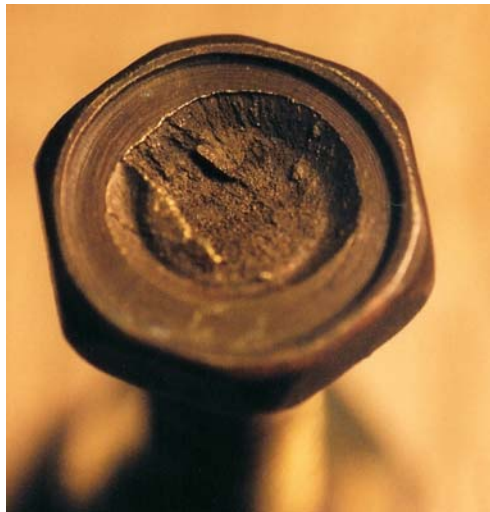
Figure 8. Failure of Brass bolt.
