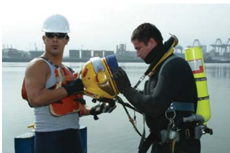
Divers should always wear a bail-out bottle, no matter what the water depth.
