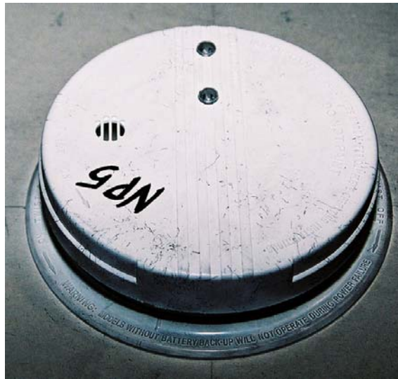
Figure 11 – Non-powered Kidde Smoke Alarm without Acoustic Soot Agglomeration on the sound exit grillwork
