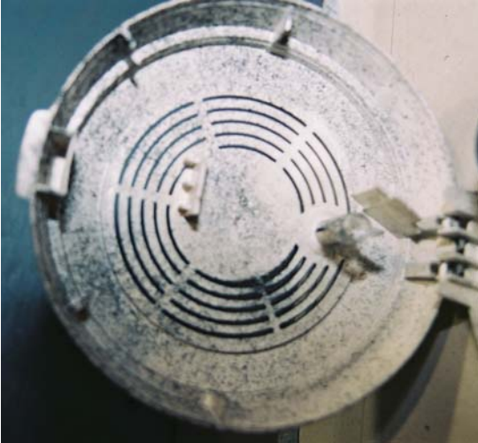
Figures 12a. and b. - Acoustic Soot Agglomeration on the interior surface of the smoke alarm case directly over the horn compartment central sound exit opening
